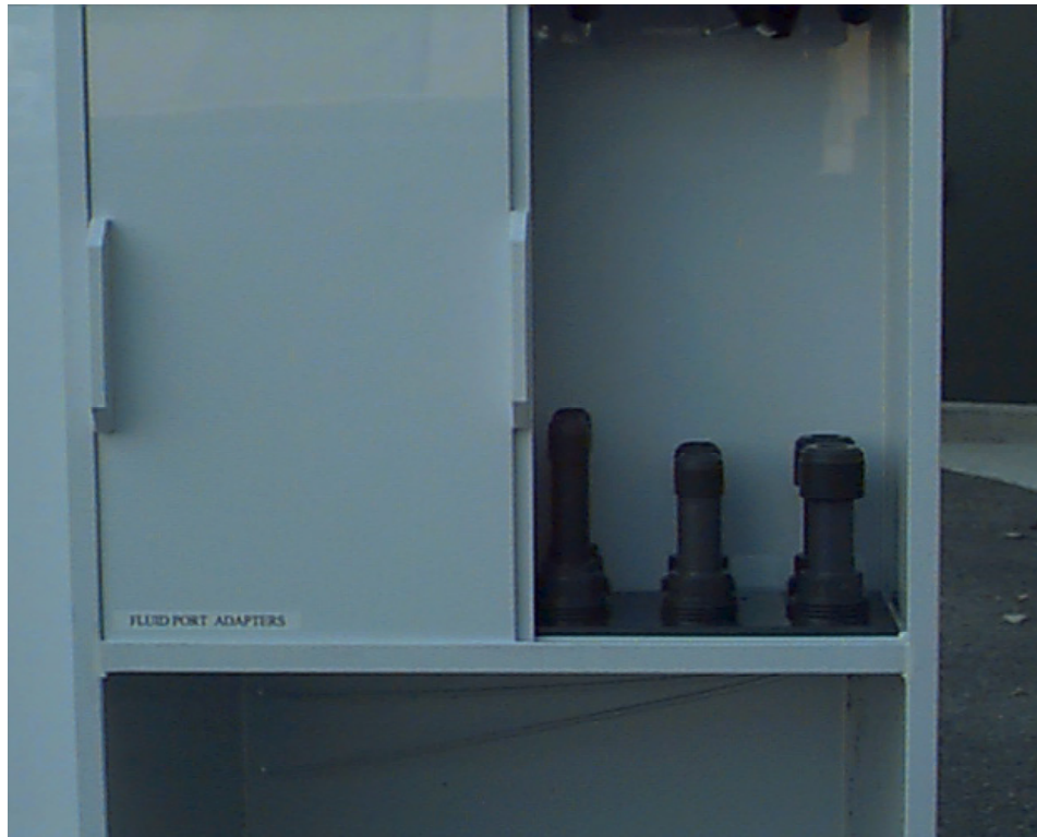
Figure 4-2: Fluid Port Adapters and Locating Plate (inside cabinet)
