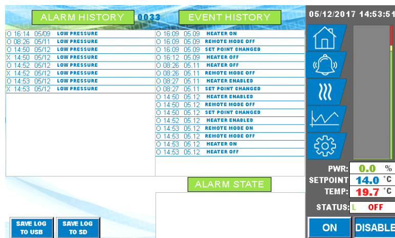
Figure 3-3: Alarm Status Page
