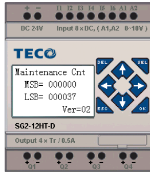
Figure 6: Maintenance Counter Display Page
